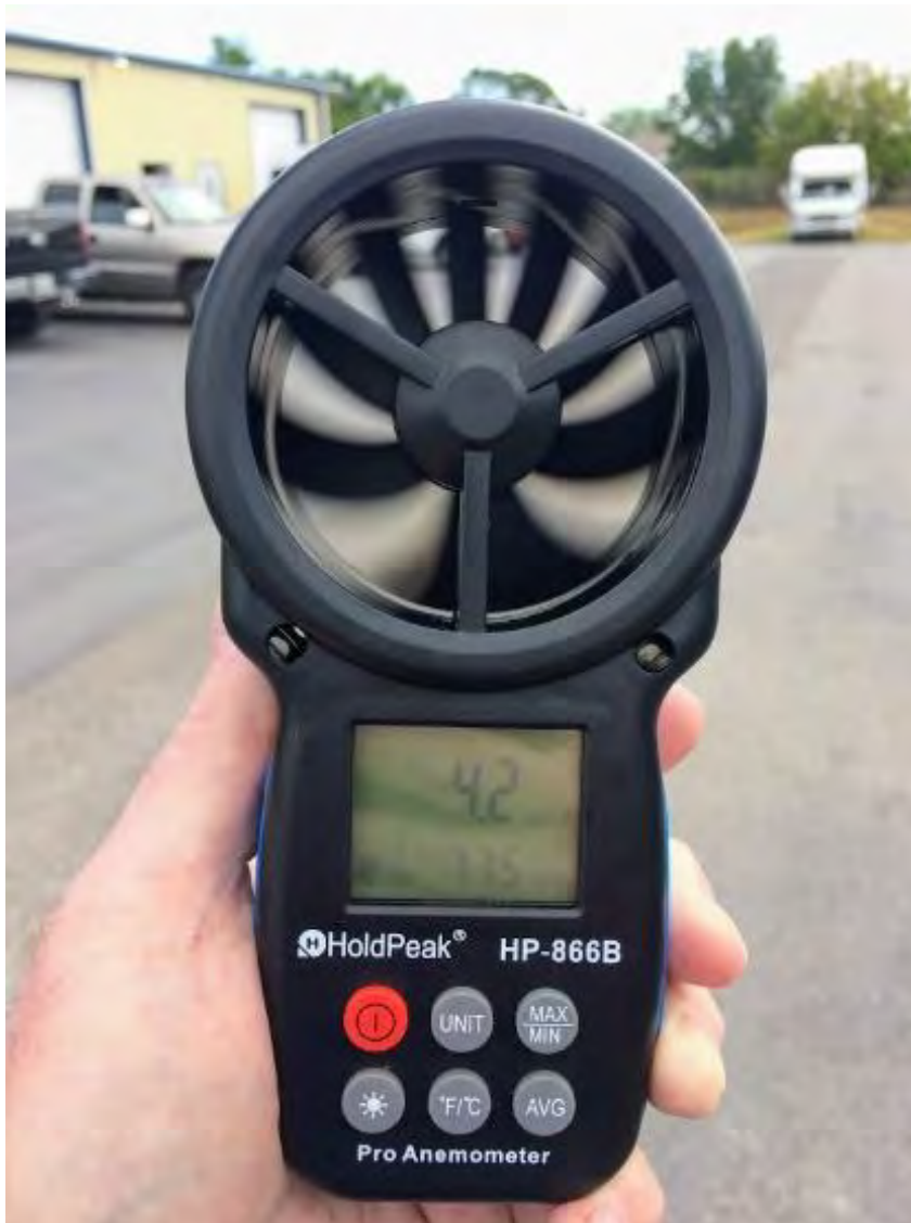
Photo 50 A handheld anemometer is useful for determining wind speeds at ground level; however, it cannot determine windspeeds above the discharge site or other locations around a display site. The larger the aerial shells, the larger the display site and the higher the bursts in the sky, making wind speed and direction both more critical and more difficult to assess in order to conduct a safe Show
