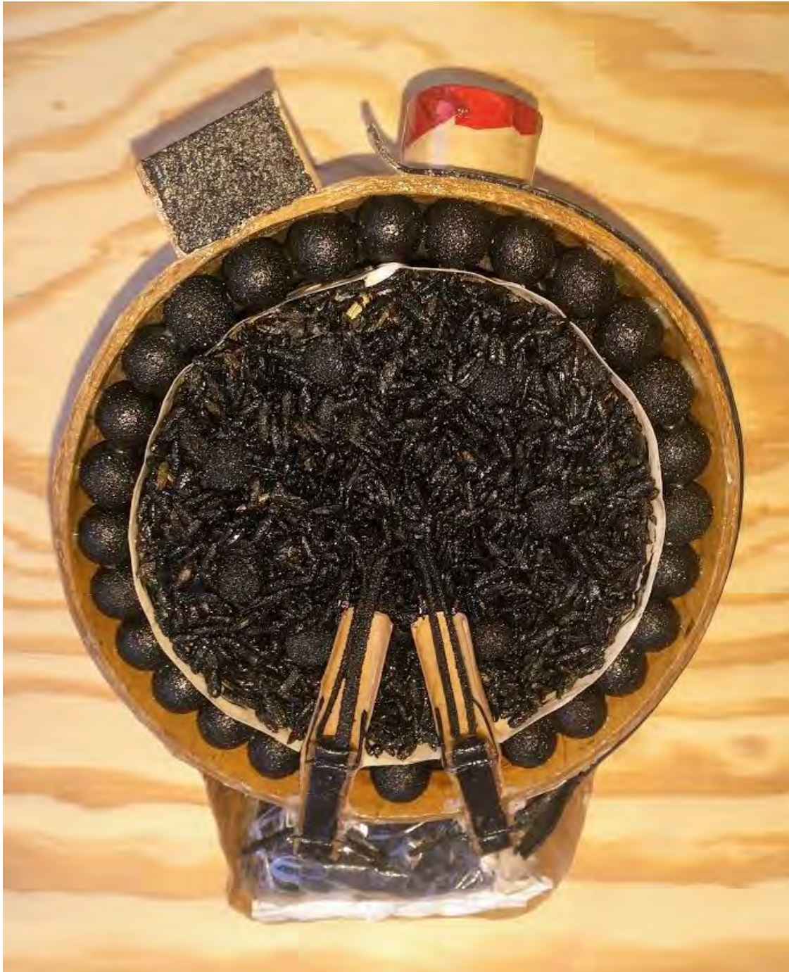
Photo 51 A cutaway of a Chinese 6" single break peony with a pistil and rising tails shell. The leader fuse fits through a string loop at the top to the lift charge of black powder in a plastic bag at the bottom. Two time fuses with crossmatch are glued into place through the paper casing from the lift charge to the burst charge in the center, which consists of dry rice hulls coated with black powder. The smaller round stars in a circle inside the burst are the pistil round stars are the petals of the peony. The rising tails are glued on the outside top of the casing and ignited by the lift charge.
