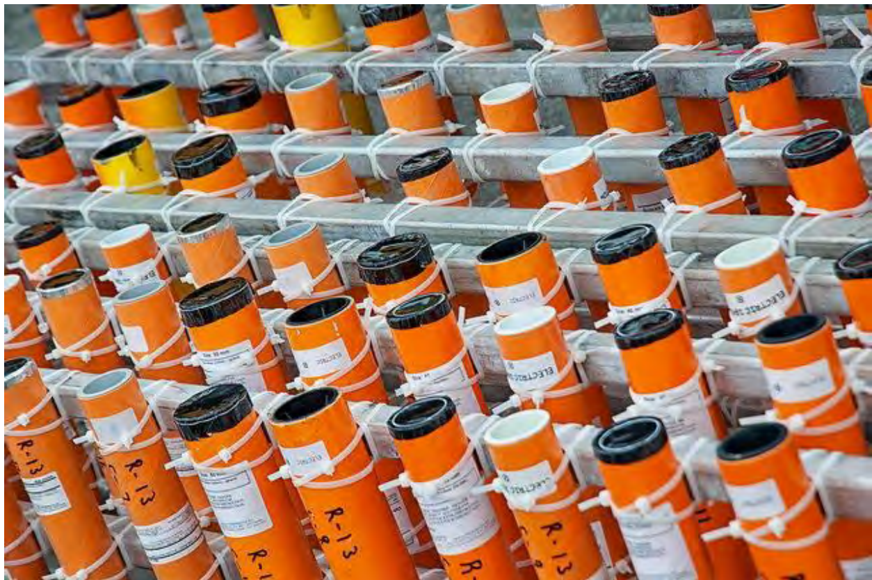
Photo 55 An example of dozens of “Single shots” secured to metal holders with nylon wire ties. Single shots are a cardboard tube with a single aerial shell, mine or comet. They can either be display fireworks
