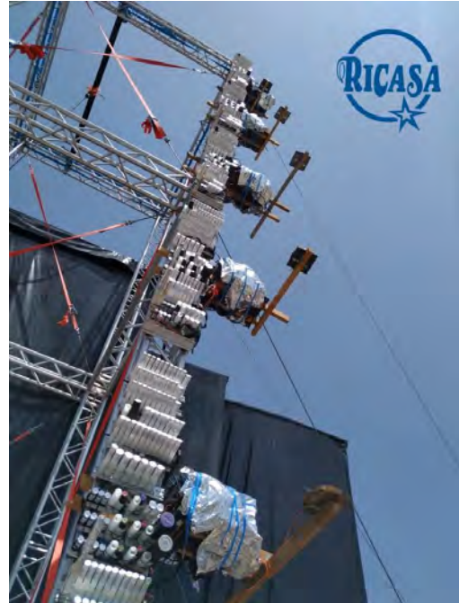
Photo 22 Articles pyrotechnic in metal holders and mounted on a truss. Article pyrotechnic are typically light enough and have low recoil so they can be placed in metal holders that can be mounted to almost any sturdy structure. [Photo credit: Pirotecnia Ricardo Caballer S.A.]
