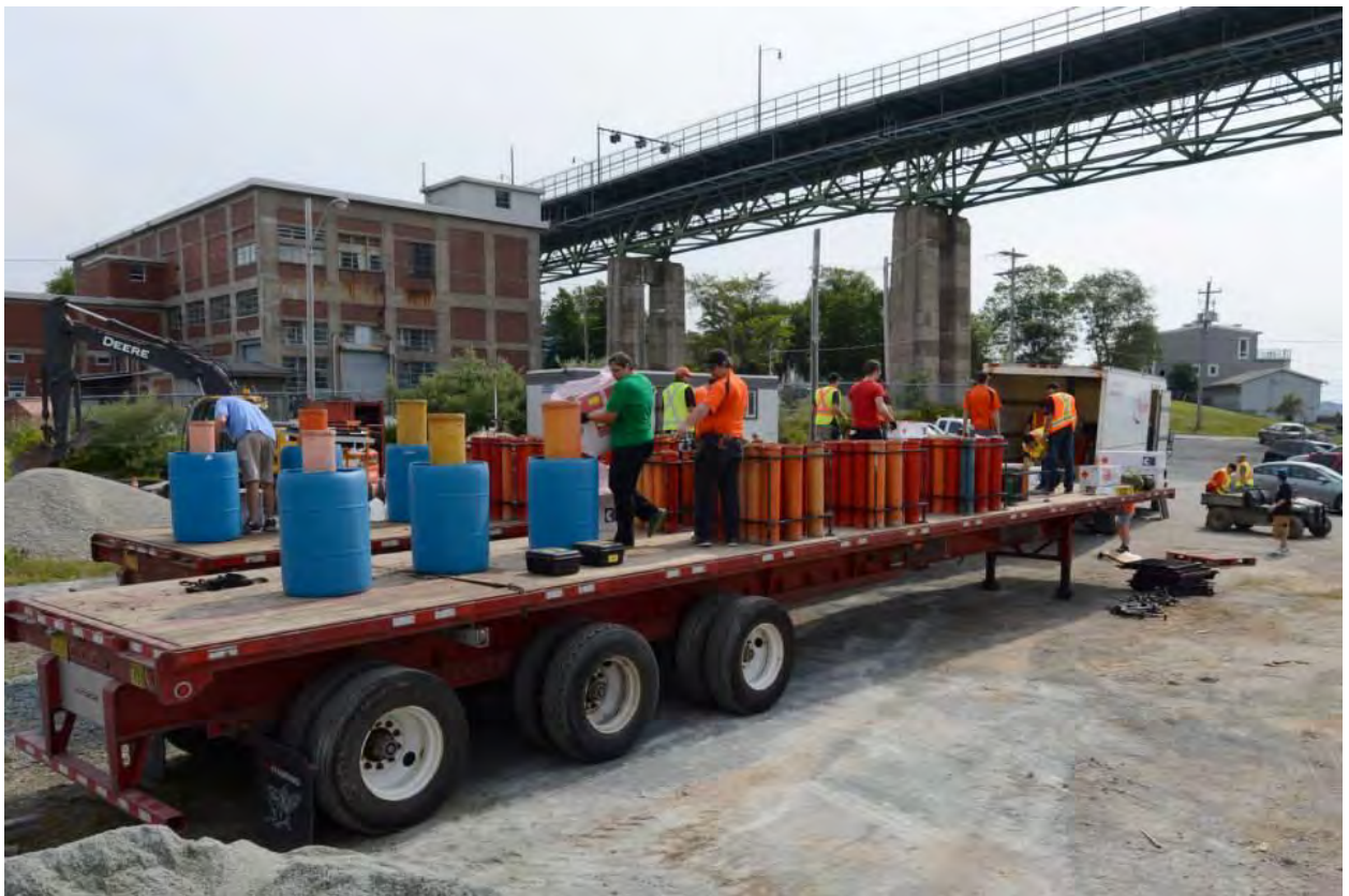
Photo 29 Two flatbed trailers with drums filled with sand for large diameter mortars and heavy-duty metal frame racks for medium diameter mortars. A trailer or dumpster can be setup and the fireworks loaded at a secure location, and then the roads closed to the public for movement of the trailer or dumpster to the discharge site on the day of the show. [Photo credit: Fireworks FX, Inc]
