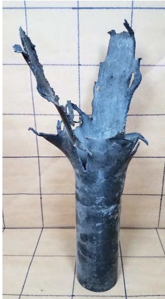
Photo 13 A 3" blowmolded HDPE mortar after a 3" single break salute shell was intentionally burst in the mortar. Note how the HDPE has stretched before failing in the classic banana peel deformation.
