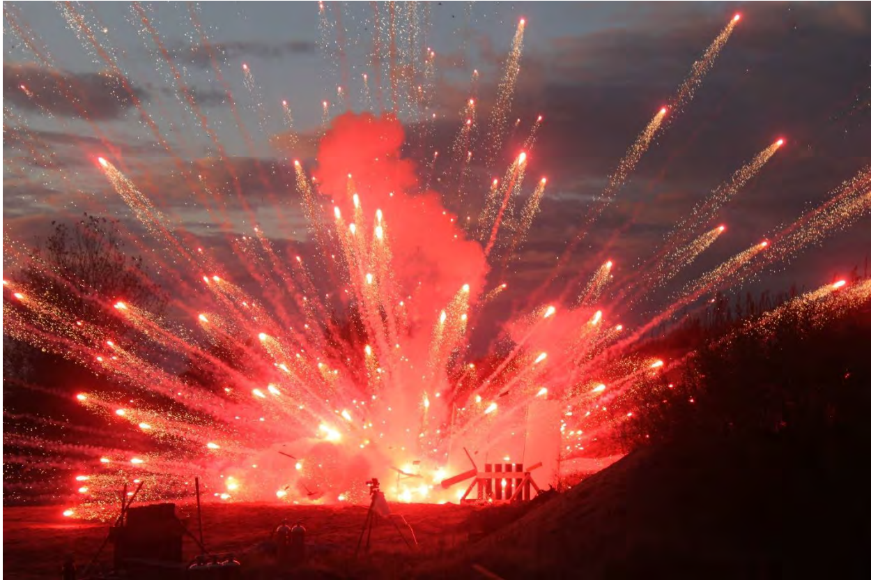
Photo 9 An example of a catastrophic aerial shell malfunction in a mortar. A 6" single break color shell has just burst inside a 6" HDPE mortar with a wood plug in an above ground wood frame rack. This photo was taken from over 100 feet away. Note an HDPE mortar from the mortar rack and pieces of the mortar rack flying up and out from the explosion with the fireball of the burst charge and burning stars, some of which landed still burning over 200 feet away.
