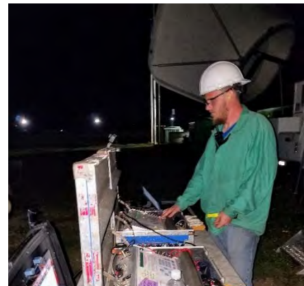
Photo 42 The Shooter, who is the Operator for this fireworks display, controlling three computer firing panels as well as a computer with the music and the time code to the computer firing panels. This fireworks display has just under 1,000 cues with 1,400 fireworks devices and over 10,000 shots fired in 20 minutes to music.
