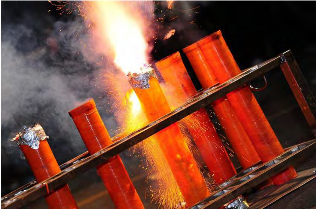
Photo 49 An example of a heavy duty above ground metal frame rack with medium level mortars. Here a shell as just fired electrically from a Chinese fiberglass mortar Note: The sparks on the outside are from the leader fuse and the light of the lift charge illuminates the inside of the fiberglass mortar. This type of rack can withstand a catastrophic malfunction in a mortar from single break color shells. [Photo credit: Fireworks FX, Inc]
