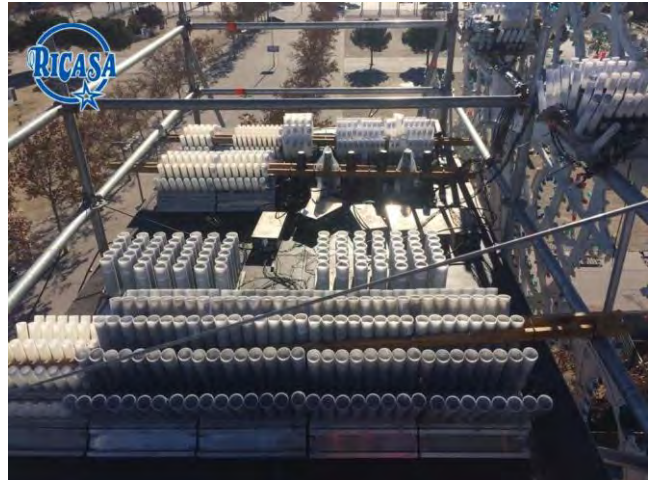
Photo 23 Article pyrotechnic in metal holders placed on top of a truss. These smaller mine and comets effects can be as dramatic or even more dramatic than aerial shells, yet they can be placed in many locations not suitable for mortars and much closer to the spectators. They also have almost no fallout and thus present less hazard to any nearby combustible materials. [Photo credit: Pirotecnia Ricardo Caballer S.A.]
