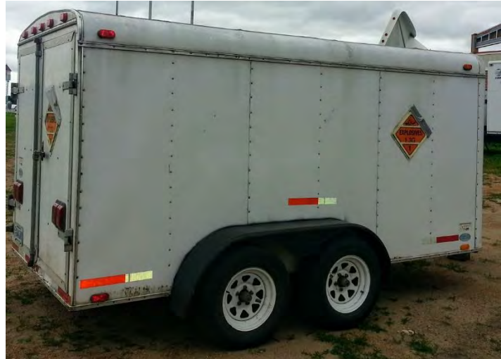
Photo 46 Temporary fireworks storage prior to the show setup can be as simple as a truck or trailer that complies with the US DOT requirements for transportation and ATF requirements for temporary storage. It must be located in a secure area away [the distance will depend on the quantity of fireworks] from occupied buildings and public roads, along with other requirements to secure the vehicle from unauthorized movement.
