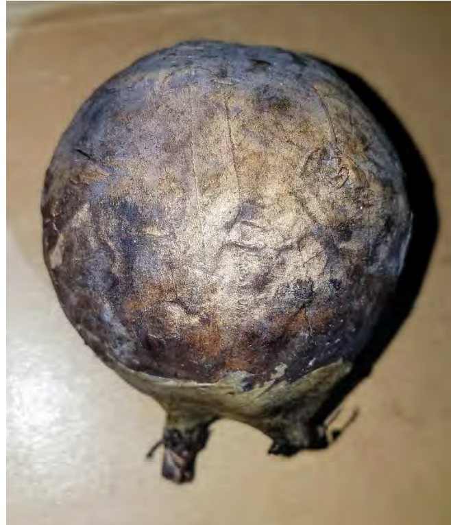
Photo 53 A 4" dud shell. Note the two times fuses on the bottom that both failed to transfer fire from the lift charge to the burst charge inside the shell. Duds are difficult to find in the dark, even in an open field of short grass. They are even more difficult to find in a pine forest on steep, rock mountains.
