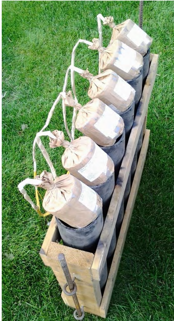
Photo 56 A rare sight at a 21 st Century Independence Day fireworks displays. An entire 4" mortar rack with American manufactured canister (cylindrical) aerial shells. Note how this rack is staked individually to the ground for support and the aerial shells are chain fused.
