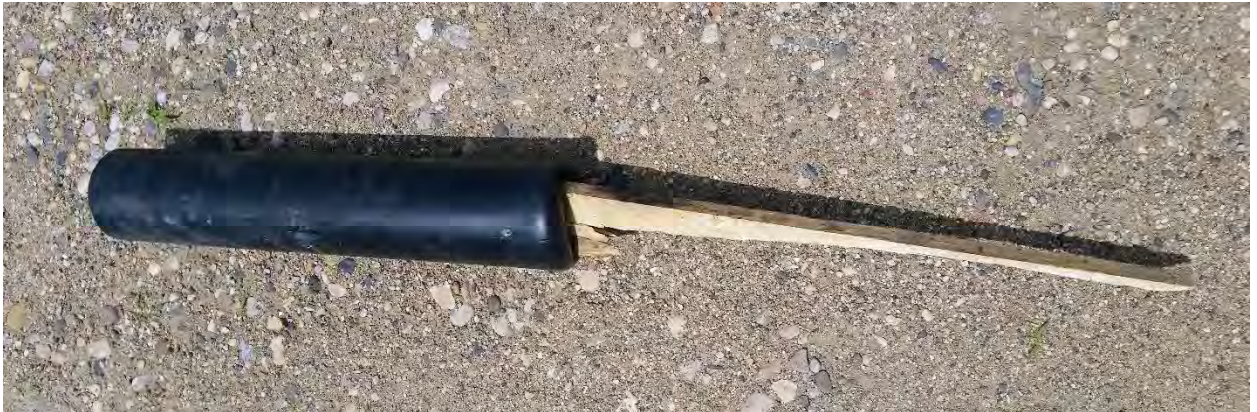
Photo 60 A 3" blowmolded HDPE mortar with the shattered remnant of a 1" x 4" sideboard from an above ground wood frame mortar rack. This large splinter is piercing the bottom of the HDPE mortar, which gives an indication of the power of 3" salutes when there is a catastrophic aerial salute malfunction in a mortar.
