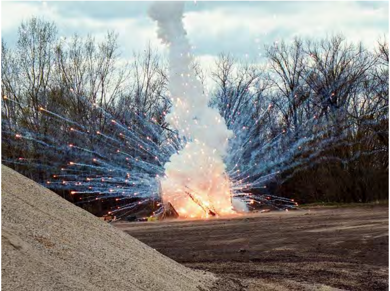
Photo 37 A 4" catastrophic aerial shell malfunction in a cardboard mortar. This single break color shell has destroyed the above ground wood frame mortar rack and the sandbags that were used to brace it. Note the entire rack is coming up and out of the blast with the fireball, along with pieces of the mortar rack and the burning stars. Cakes and finale boxes with cardboard tubes, which are chain fused, will experience similar results in the event of a blowout, but because cakes and finale boxes are chain fused, they likely will continue to fire any remaining effects at steep angles until it blows itself out, or is spent.
