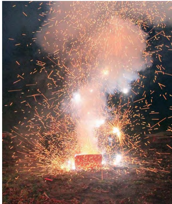
Photo 52 A cake with crackling effects being fired. Note how many of the crackling effects function in close proximity to the cake and even on the ground. Cakes can burn, which distracts from the show and creates additional risks to any nearby combustibles or property. Cakes and finale boxes can experience blowouts and continue to shoot aerial effects in all directions until it blows itself out or is spent.
