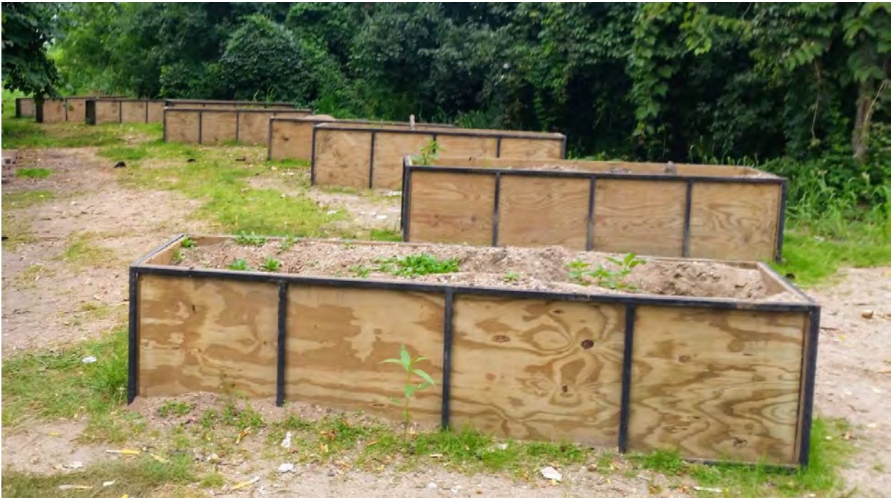
Photo 12 An example of troughs full of sand for 8", 10" and 12" mortars. Troughs and drums are often used where ground water levels are high and the soil is too soft to handle the recoil from large diameter mortars, or where the ground is too hard to bury the mortars.
