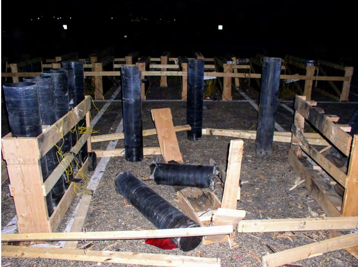
Photo 5 An example of a catastrophic aerial shell malfunction in a mortar. An 8" aerial shell functioned prematurely in an American made fiberglass mortar with a wood plug screwed into the bottom. The mortars were mounted in above ground wood frame racks.
