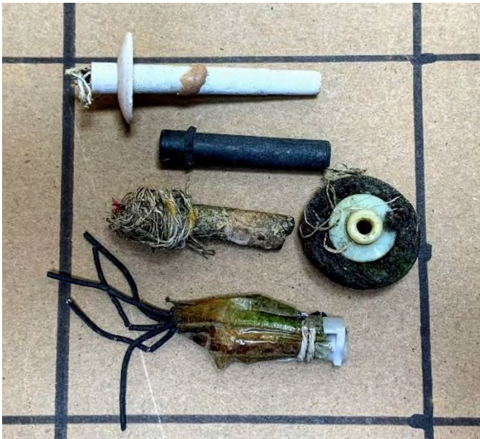
Photo 17 Some of the plastic debris recovered in the Hall of Records during the survey of October 2019, ten years after the last fireworks display. These are a plastic time fuse tube from a large diameter aerial shell, plastic time fuse holders from medium diameter aerial shells, a spacer with a plastic time fuse holder from a Roman candle, and the remnant of a quickmatch leader fuse in a plastic casing with a plastic T connector for an electric match (Note the strands of still viable blackmatch fuse)
