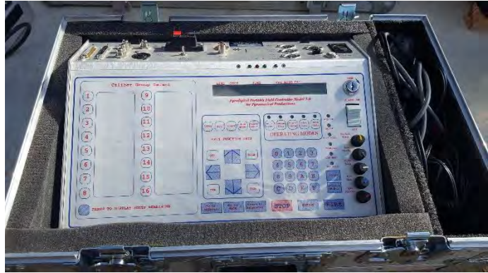
Photo 8 An example of a computer firing control panel. These panels can fire thousands of cues in increments as fast as 1/10 th of a second. They are proprietary and together with the design software, testers, junctions, firing modules and cables needed to make the entire system work, can cost tens of thousands of dollars
